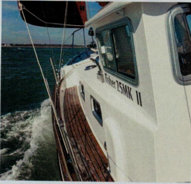
ABOVE Deep bulwarks and plenty of handholds as you move forward along the side decks
