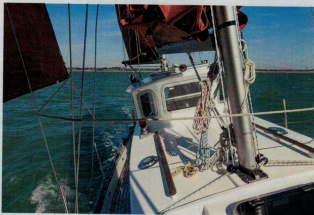
ABOVE The tiller is stowed on the aft side of the wheelhouse, ready to be shipped if you need or want to helm from the cockpit
